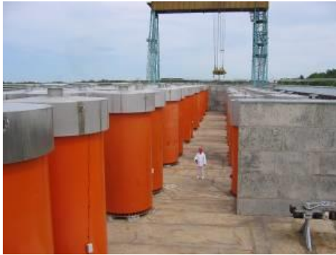
The dry RBMK-1500 spent fuel cask storage site at the Ignalina NPP (Lithuania)
